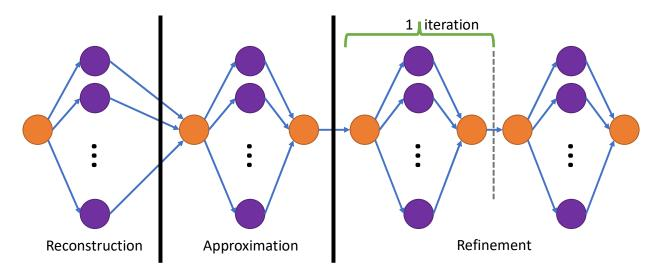
Figure 7.4: APT's highly-parallel fork-join GRB localization task.
