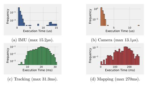
Figure 5.10: ORB-SLAM3 task execution time distributions.
