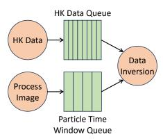
Figure 5.6: The FIMS Computational Pipeline
