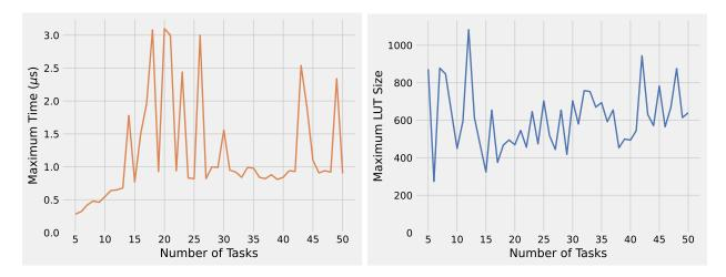
Figure 5.16: Maximum LUT sizes and times to perform binary search for each number of tasks.
